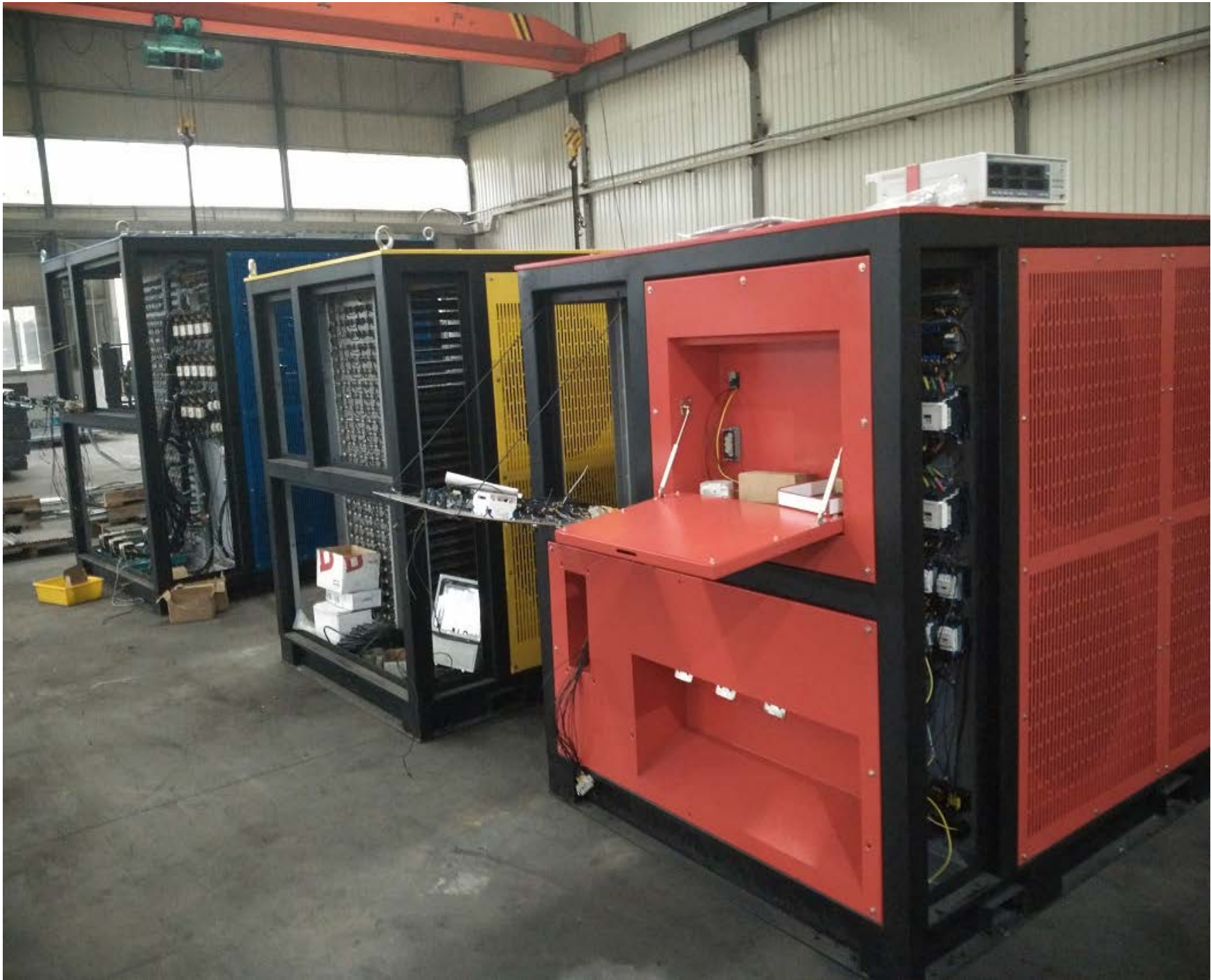
Load Bank to Test Gensets
